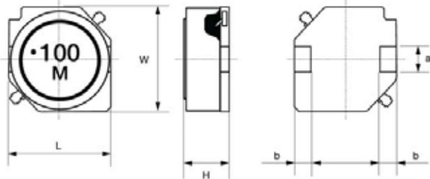
※ The NS 101□□ type does not have the indication of the Manufacturing date code.
